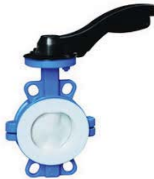
INDUSTRIAL SPLIT BODY BUTTERFLY ONE-PIECE DISC/STEM DESIGN BI-DIRECTIONAL "U" QJP STEM SEAL SIZES: 2"-24" MATERIAL: SS, CAST IRON, BUNA/ EPOXY, TFE LINED
