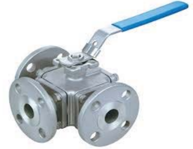
3WAY FLANGED BALL VALVE DIRECT MOUNT DESIGN FULL & STANDARD PORT SIZES: 1/2" - 6" MATERIAL : CARBON/STAINLESS ANSI 150,300,600#
