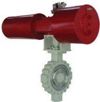
HIGH PERFORMANCE TRIPLE OFFSET METAL SEATED/ SOFT SEATED ZERO LEAKAGE AND TIGHT SHUT-OFF TRIPLE ECCENTRIC DESIGN SIZES: 3"-24" MATERIAL: CARBON/ STAINLESS STEEL LUG/WAFER BODIES
