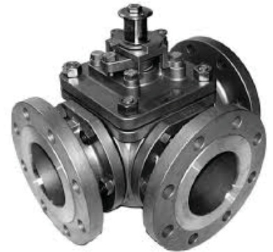
3 WAY TYPE L - T PORT VALVES BI-DIRECTIONAL ANSI 150-600#RF FLANGED SIZES: 2"-24" MATERIAL: CARBON/STAINLESS STEEL
