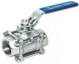
3 PC FOUR BOLT 1000 PSI BALL VALVE CONNECTION TYPE: NPT, SOCKET SIZES: 1/2" - 4" MATERIAL: CARBON, STAINLESS STEEL
