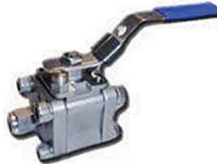
3-PC 4 BOLT CONCEALED 2000 PSI BALL VALVE CONNECTION TYPE: COMPRESSION SIZES: 1/4" - 1" MATERIAL: CARBON/ STAINLESS
